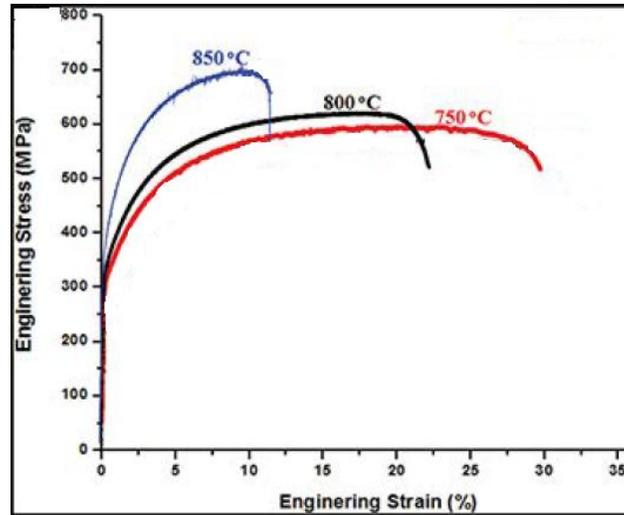
Fig 3:- Stress-strain curves for DP-steel specimens annealed at various temperature time conditions under controlled cooling.
