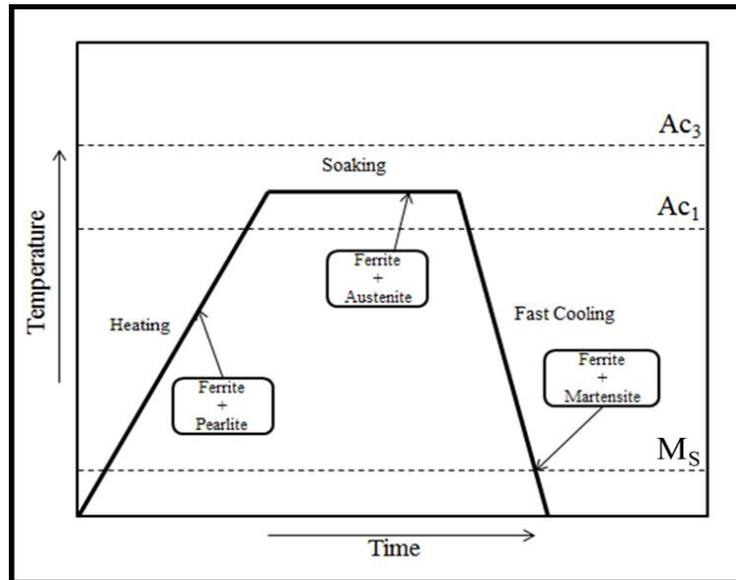
Fig. 1 Schematic for phase transformation during heating, holding and cooling of DP steels[13]
