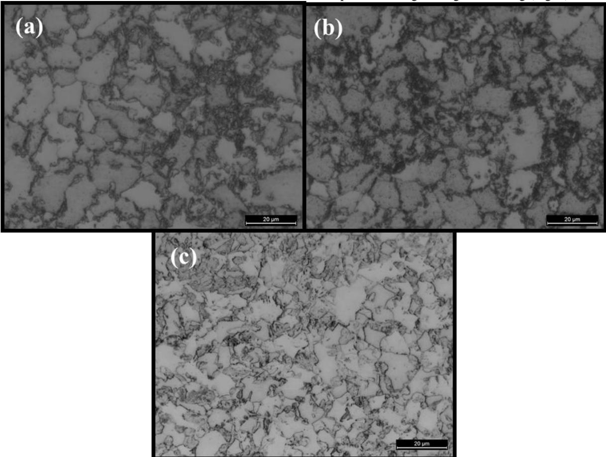
Fig2: Optical micrographs of DP-steel samples annealed in annealing simulator at various temperature and for 3 min soaking time (a) 700  $^{\circ}\text{C}$  (b) 800  $^{\circ}\text{C}$  (c) 850  $^{\circ}\text{C}$
