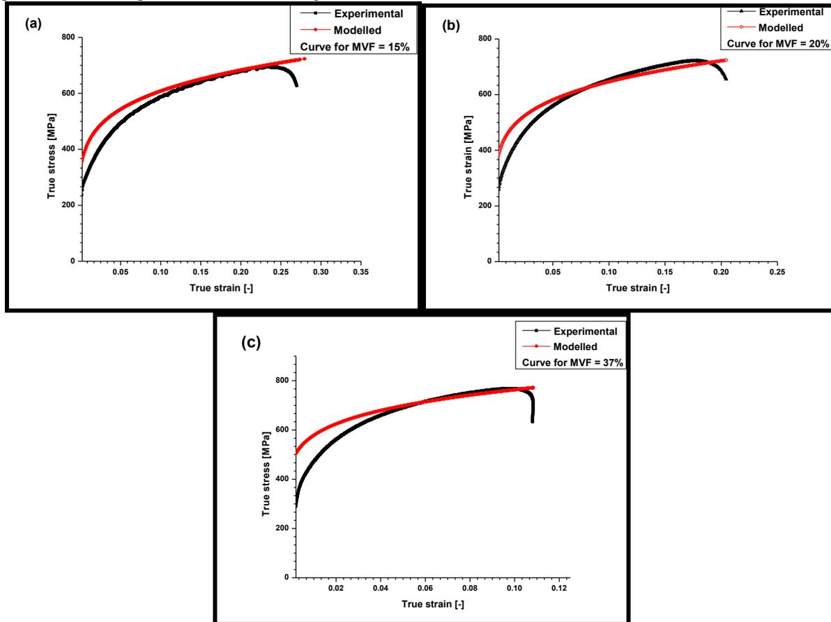
Fig. 5: Comparison of experimental and modelled true stress strain curves of DP-steel for different MVF (a) 15% (b) 20% (c) 37%. MVF = Martensite volume fraction
