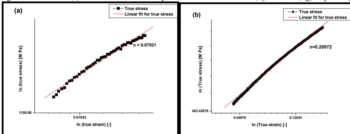
Fig. 4: ln-ln true stress-strain curves of DP-steel to obtain strain hardening exponent for (a) martensite and (b) ferrite
